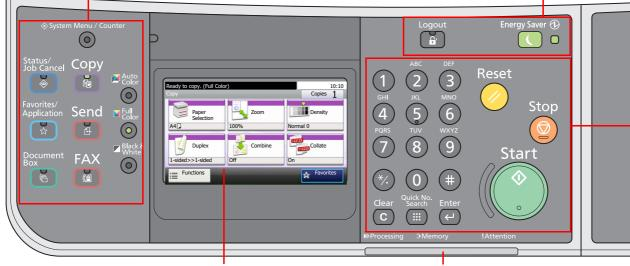
Touch panel. Displays buttons for configuring machine settings.
