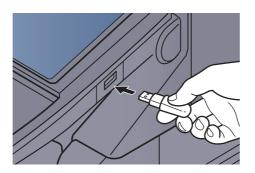
When the machine reads the USB memory, "Removable Memory is recognized. Displaying files. Are you sure?" may appear. Press [Yes] to display the removable memory screen.
