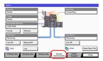
The screen to check the status or configure the devices is displayed.
