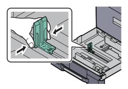
2 Press the (Paper Width Guide) Lock to release the lock. Grasp the paper width adjusting tab and move the paper width guides to fit the paper.
