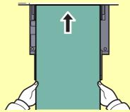
After printing starts, catch the paper when it is output so that it does not fall. When using the inner tray as the output location, do not stand up the stopper.
