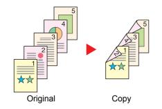
Produces two-sided copies from one-sided originals. In case of an odd number of originals, the back side of the last copy will be blank.
