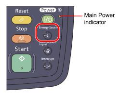
If print data is received during Low Power Mode, the machine automatically wakes up and starts printing. Also when fax data arrives while the machine is in Low Power Mode when using the optional fax, the machine automatically wakes up and starts printing.
