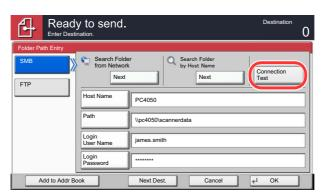
"Connected." appears when connection to the destination is correctly established. If "Cannot connect." appears, review the entry.
