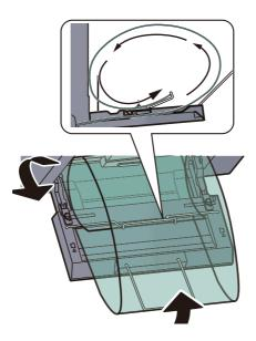
4 Adjust the paper width guides to the width of the paper.
