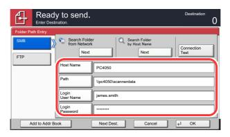
2 Press [Connection Test] to check the connection.
