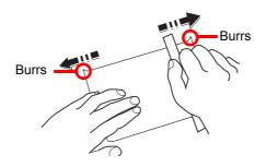
Before loading Hagaki into the multi purpose tray, fan them and align the edges. If the Hagaki paper is curled, straighten it before loading. Printing onto curled Hagaki may cause jams.
