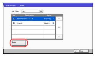
"Status/Destination" is displayed when address is selected. Press [Detail] to display the list. Press [ $\checkmark$ ] or [ $\land$ ], select a destination and press [Detail]. Information on the selected job is displayed for checking.
