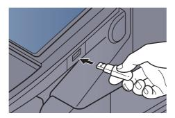
When the machine reads the USB memory, "Removable Memory is recognized. Displaying files. Are you sure?" may appear. Press [Yes].
