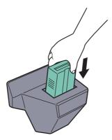
Insert the key counter securely into the key counter slot.
