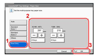
If you select [Size Entry], press [+], [-] to enter "X" (horizontal) and "Y" (vertical) dimensions. By pressing [# Keys], you can use the numeric keys.
