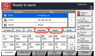
Select a destination and press [Detail/Edit] to check and edit it. Edit the delay as required. Select a destination and press [Delete] to remove the destination from the list.
