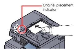
Put the side to be scanned (or the first side of two-sided originals) face-up. Slide the leading edge into the document processor as far as it will go. The original loaded indicator lights when the original is placed correctly.
