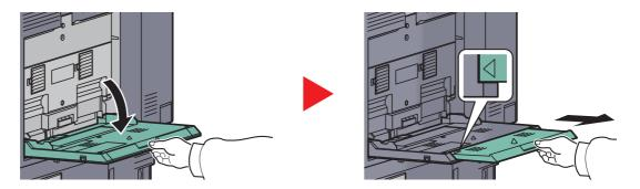
When loading paper sizes 12 x 18" and from A3 to B4 and Ledger to Legal, extend the support tray section of the multi purpose tray until the " $\Delta$ " mark is fully appeared.
