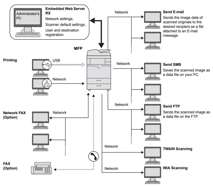
TWAIN and WIA are standardized interface for communication between software applications and image acquisition devices.
