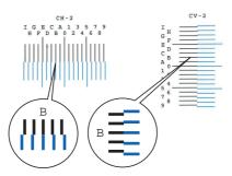
Find the location on each chart where 2 lines most closely match. If this is the 0 position, registration for that color is not required. For the illustration, B is the appropriate value.
