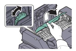
If the original is difficult to remove, turn the dial. The original will scroll out to a position where it can be removed easily.
