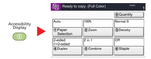
You can also control the screen using the numeric key corresponding to the number in circle. (Example: Press the [2] key on the numeric key pad to zoom.)
